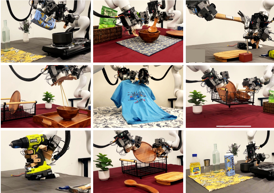
Figure 1: Bimanual Dexterity: BiDex can effortlessly teleoperate various complex tasks including pouring, scooping, hammering, chopstick picking, hanger picking, picking up basket, drilling, plate pickup and pot picking to train high-quality behavior cloning policies with over 50 degrees of freedom. Our teleoperation system and two LEAP hands [1] costs around $12k in total and is readily reproducible by academic labs.
