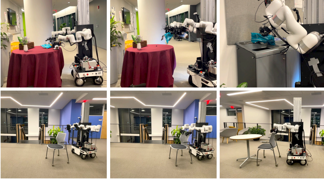
Figure 3: All Tasks : Teleoperation of the mobile robot systems with BiDex. Top : Picking up trash from a table and discarding it into a bin. Bottom : Grasping a chair and moving it to align with a table.
