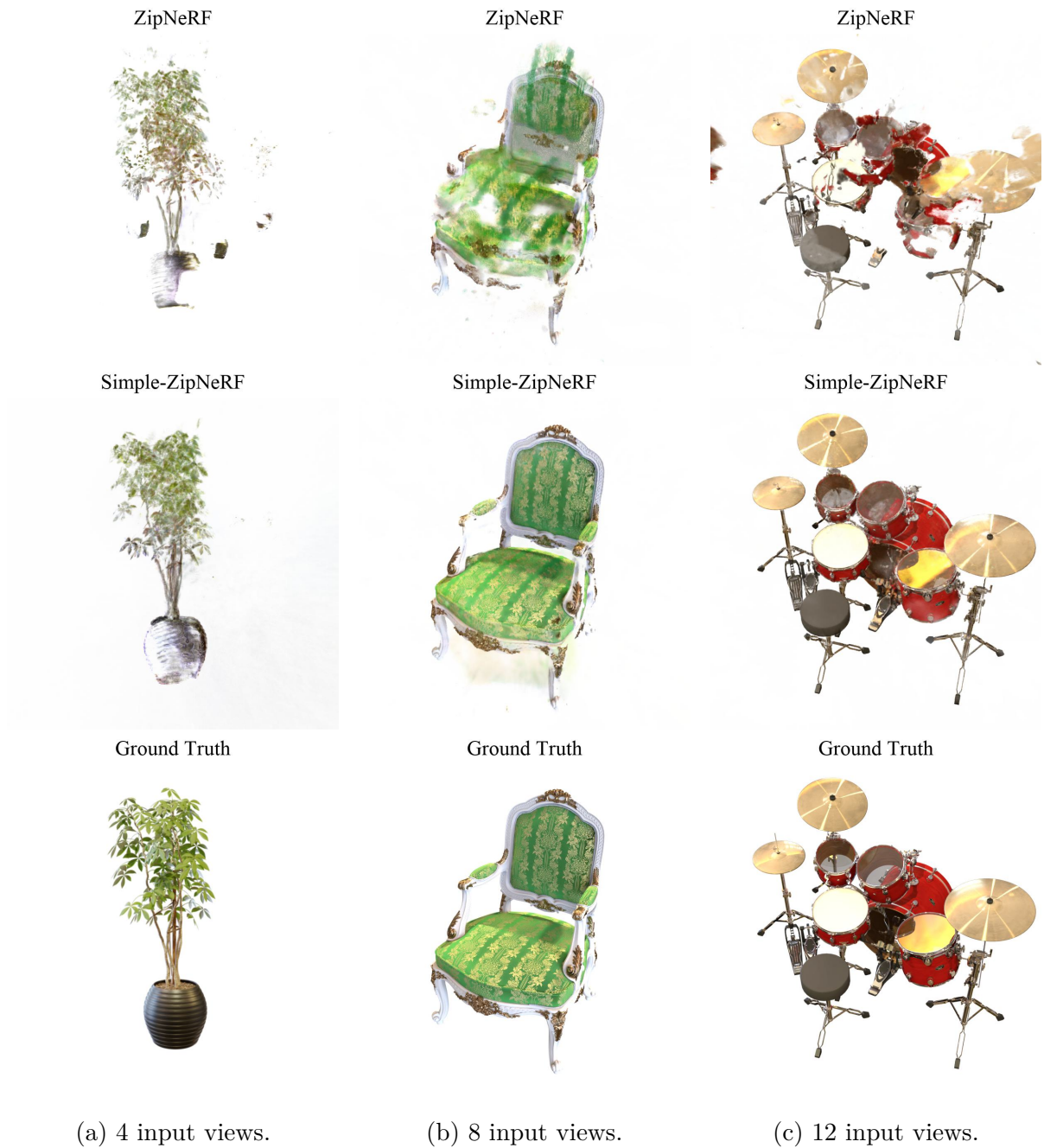
Figure 4.24: Qualitative examples of ZipNeRF and Simple-ZipNeRF on the NeRF-Synthetic dataset. While the renders of ZipNeRF contain multiple floaters, Simple-ZipNeRF outputs are cleaner and free from such artifacts.
