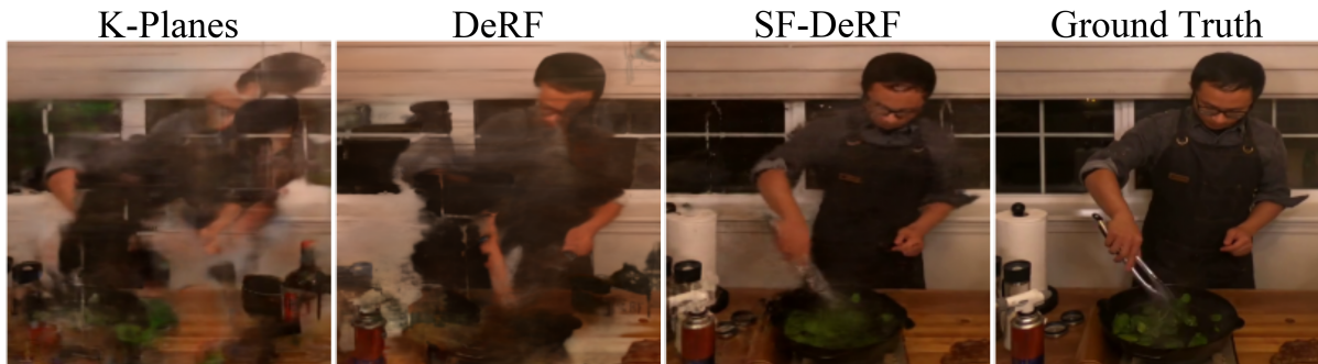
Figure 5.4: Qualitative examples on N3DV dataset with three input views: We can observe that K-Planes finds it hard to learn the moving person leading to significant distortions. Our DeRF model (without any priors) corrects a few errors by virtue of the common canonical volume. Imposing our priors leads to much better reconstruction.
