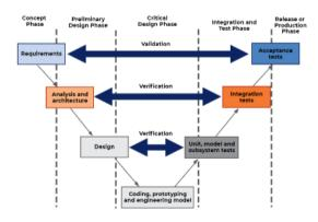
Fig. 1. V-cycle Software model
