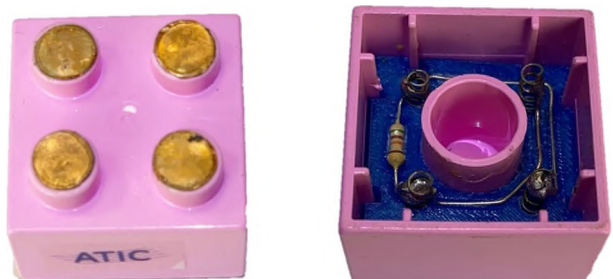
Fig. 14 Detail of modified Lego pieces employed for melody construction
