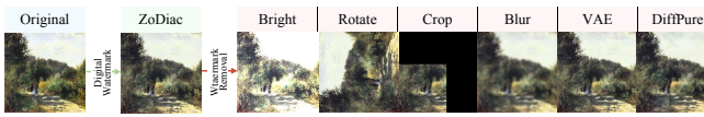
Figure 28: Fidelity visualization of DW against WR. Column 1: original image; column 2: Zodiac-watermarked image; column 3-8: watermarked images under attacks.
