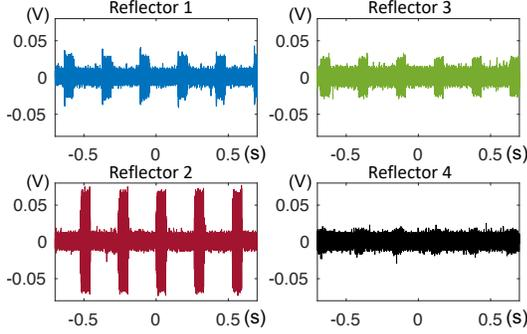
Figure 8: Received signal strength with one selected reflector programmed for 1-bit coding at a time.
