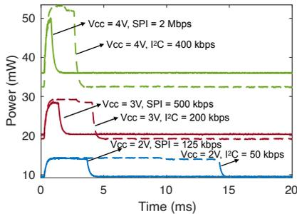
Figure 6: Power consumption of the UA-RIS at various supply voltages.
