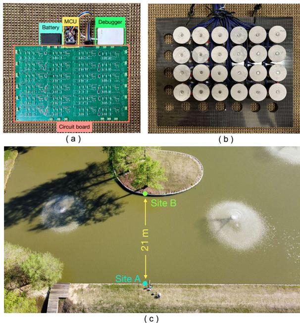
Figure 13: Lake experiments. (a) 24-channel control board. (b) Acoustic reflection units. (c) Experimental setup.
