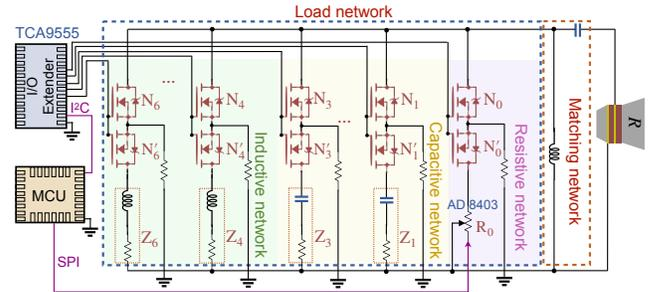
Figure 5: Architecture of the UA-RIS.
