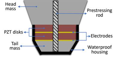
Figure 4: Tonpiliz reflector used in our UA-RIS.
