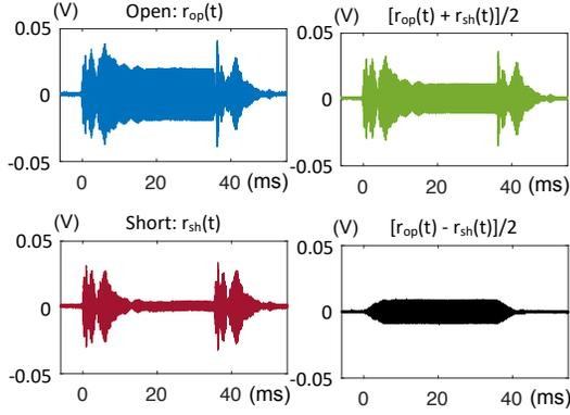
Figure 10: Waveform comparison of received signals with and without the reflector.
