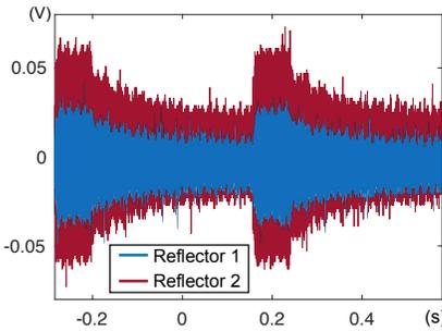
Figure 9: Variation in strength of the received signal with changes in potentiometer's resistance.
