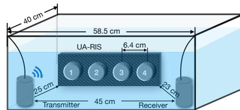
Figure 7: Settings of tank tests.
