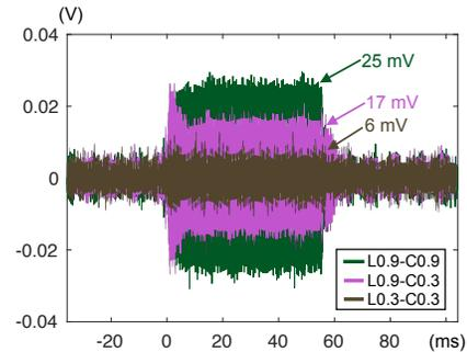
Figure 12: Differential signal with inductive and capacitive loads at the acoustic reflector.
