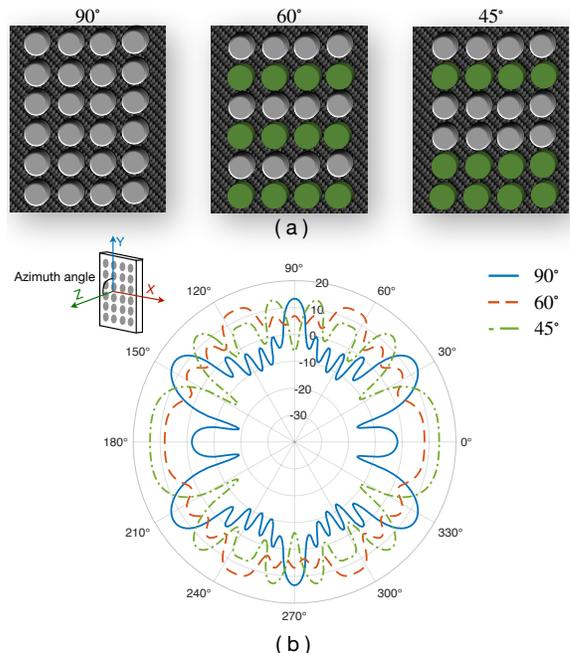
Figure 14: Load configuration of UA-RIS for beamforming at the transmitter side. (a) Coding schemes for steering. (b) Azimuth beam pattern of the reflected waves.
