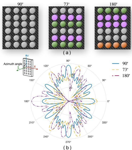
Figure 16: Load configuration of UA-RIS for beamforming at the receiver side. (a) Coding schemes for steering. (b) Azimuth beam pattern of the reflected waves.
