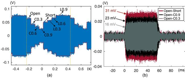
Figure 11: Waveform of the received signal with variations in load impedance. (a) Original waveform. (b) Differential waveforms.
