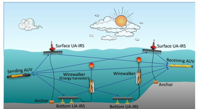
Figure 2: UA-RIS assisted long-range underwater acoustic communication network.
