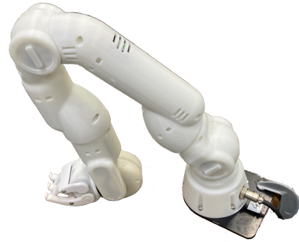
Fig. 5. CRANE-X7 manipulator with a cross-structured hand.
