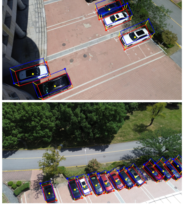
Figure 8. Illustration of the 3D bounding box are obtained by Coordinate System Transformation.
