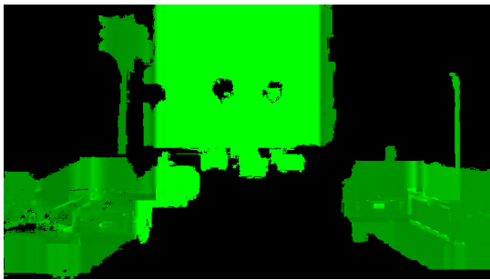
Fig. 9. A decoded Delta-frame exhibiting corruption caused by simulated packet loss. The background, represented by black pixels, remains unchanged as the positions of corrupted masks are transmitted in the form of polygons.
