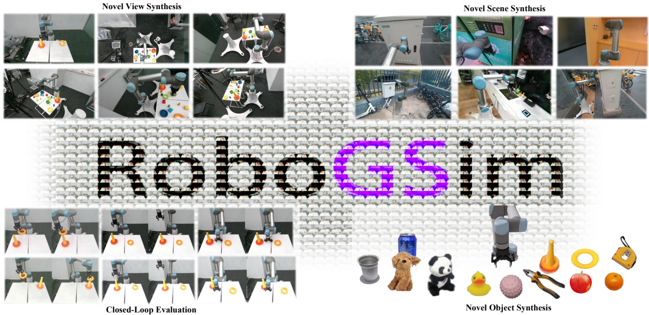
Figure 1. RoboGSim is an efficient, low-cost interactive platform with high-fidelity rendering. It achieves demonstration synthesis with novel scenes, novel objects, and novel views, facilitating data scaling for policy learning. Additionally, it can perform the closed-loop simulation for safe, fair and realistic evaluation on different policy models.
