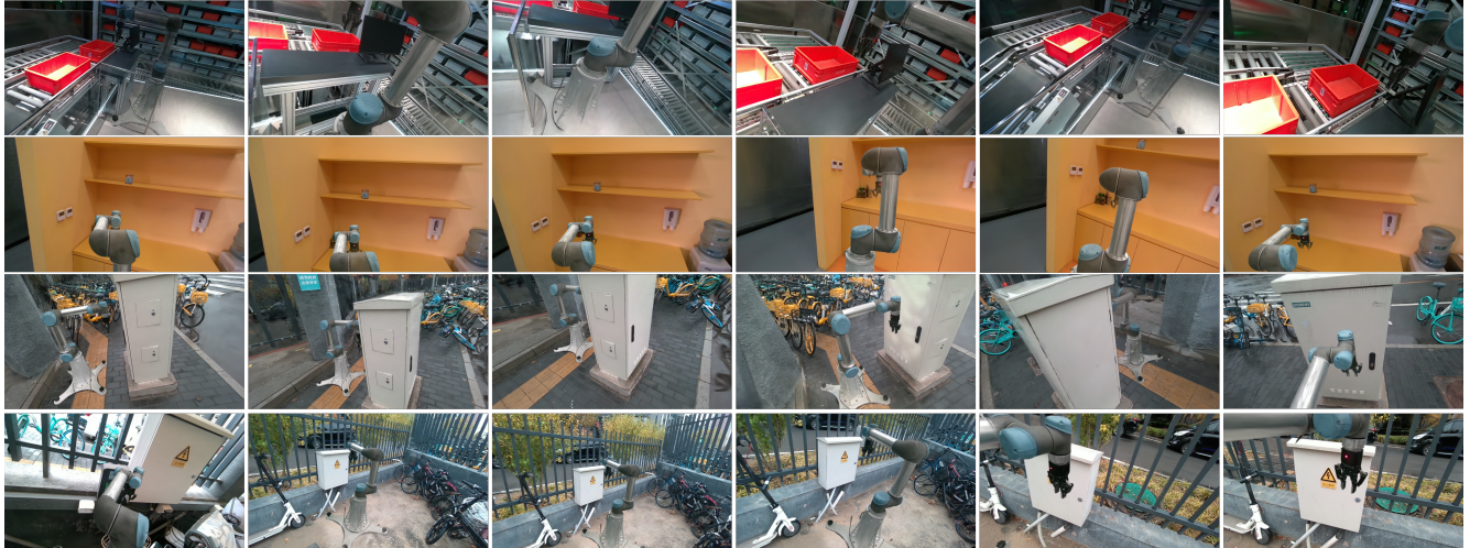
Figure 5. Novel Scene Synthesis: We show the results of the physical migration of the robot arm to new scenes, including a factory, a shelf, and two outdoor environments. The high-fidelity multi-view renderings demonstrate that RoboGSim enables the robot to operate seamlessly across diverse scenes.
