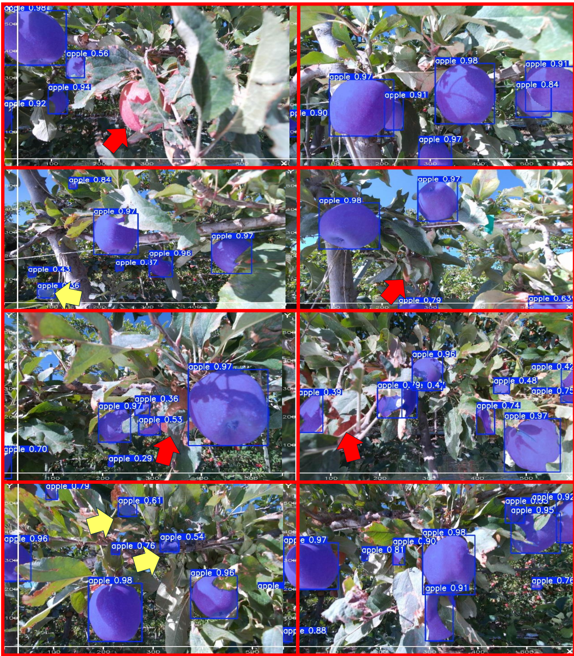
Fig. 11: Showing the examples of the efficacy of our zero-shot learning-based instance segmentation model on commercial apple orchards, with a Microsoft Azure machine vision camera. This figure demonstrates the model’s performance, trained solely on LLM-generated and SAM-annotated synthetic datasets. Red arrows highlight regions where occluded apples were not segmented due to complex environmental factors, while yellow arrows show false positive segmentations of canopy foliage as apples. These visual outcomes emphasize the model’s potential and the need for enhanced data realism and volume to improve accuracy in real-world applications.
