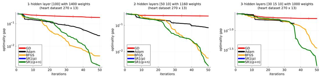
Figure 2: Using negative step sizes in training neural networks. The plots show training error by iteration for neural networks with 1-, 2- and 3- hidden layers on the `heart` dataset. We compare full QN methods BFGS (yellow) and SR1 (blue and green) with GD (red) and Adam (black). SR1 is non-convergent with positive-only step sizes (blue) but outperforms when step sizes are allowed to be negative (green). The outperformance appears more pronounced in deeper networks.
