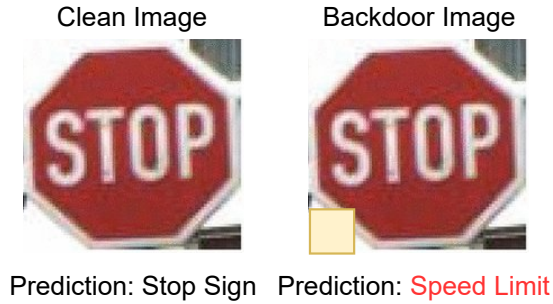
Fig. 1: Example of a backdoor image (right) and its corresponding clean image (left). A yellow square, serving as the trigger, has been added to the bottom left corner of the backdoor image.
