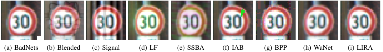
Fig. 2: Examples of different backdoor triggers used in the literature. Note that while IAB adds a local patch to each image, its position and scale can vary across images.
