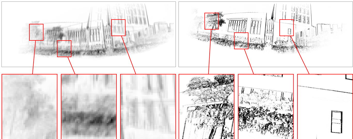
(a) CMax-SLAM result on front-gate sequence ( 1024 \times 512 resolution, empty regions trimmed), (b) EROAM result on front-gate sequence ( 2769 \times 1000 resolution, empty regions trimmed)
