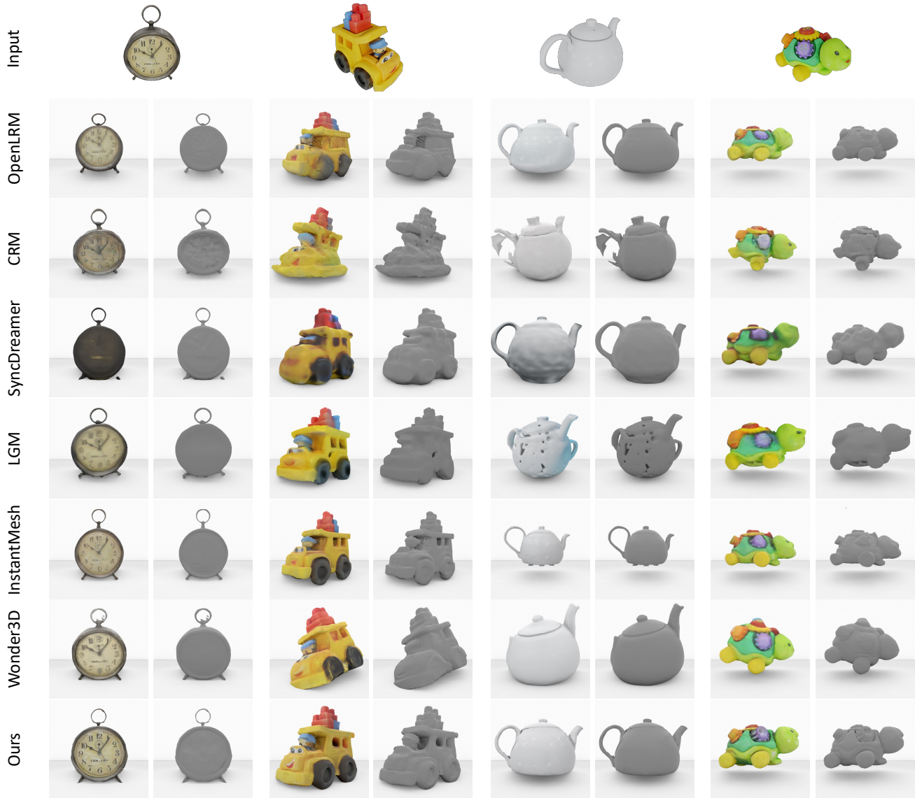
Figure 5. Qualitative results on GSO dataset. We visualize the input single image and the resulting 3D mesh (with and without textures) for our method and baselines. Our approach achieves higher mesh quality in terms of both geometry and texture.
