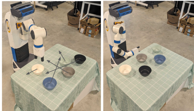
Fig. 1. An example of mobile robot tabletop rearrangement, while black arrows are the desired rearrangement goals.
