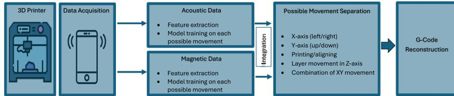
Fig. 12: Overview of the stages to reconstruct G-code
