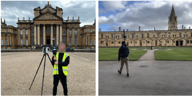
Figure 3. Leica RTC360 TLS and the Frontier device in Blenheim Palace (left) and Christ Church College (right).
