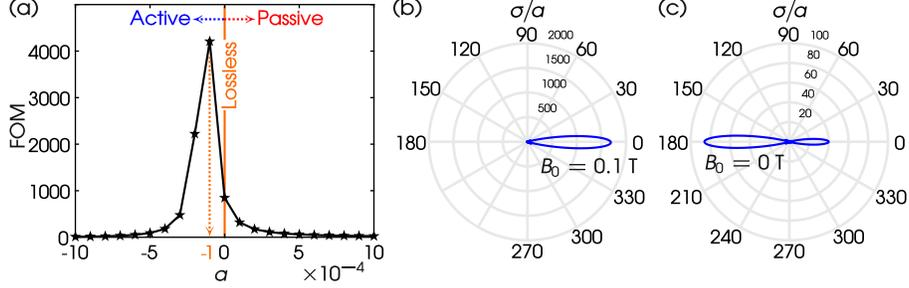
Figure 13: (a) FOM vs.  $\alpha$  for the octamer of Figure 12(a) when  $B_0 = 0.1$  T and  $f = 2.0190$  THz. (b)  $\sigma/a$  at  $\alpha = -1 \times 10^{-4}$  (active),  $B_0 = 0.1$  T and  $f = 2.0190$  THz. (c) Same as (b) but for  $B_0 = 0$  T.
