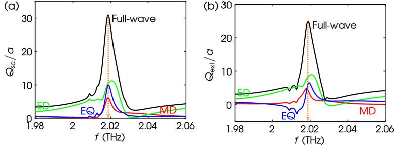
Figure 11: (a)  $Q_{sc}/a$  spectrum for the same values of parameters as in Figure 10(b) using  $\alpha = -7 \times 10^{-4}$ . Black: full-wave; red: MD; green: ED; blue: EQ. Orange dotted arrow: location of  $f = 2.0186$  THz. (b) Same as (a) but for the  $Q_{ext}/a$  spectrum.
