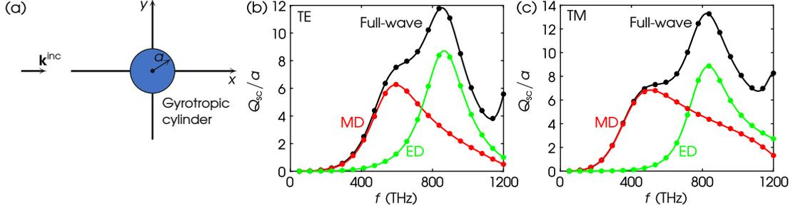
Figure 5: (a) Scattering by a gyrotropic circular cylinder. Values of parameters:  $\epsilon_{1r} = 4$ ,  $\epsilon_{2r} = 1$ ,  $\epsilon_{3r} = 5$ ,  $\mu_{1r} = 2$ ,  $\mu_{2r} = 0.5$ ,  $\mu_{3r} = 3$ ,  $a = 50$  nm. (b) TE scattering. (c) TM scattering. Curves: exact; dots: this work via COMSOL; black: full-wave; red: MD; green: ED.
