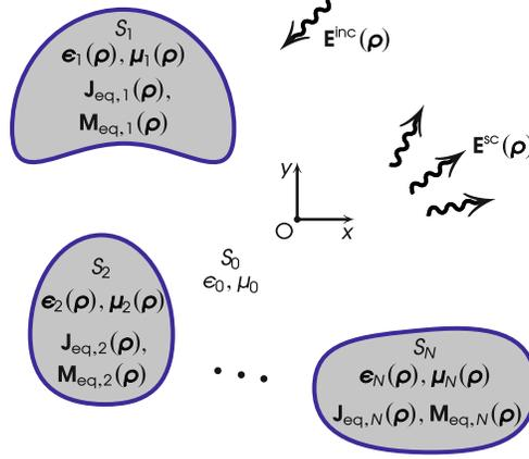
Figure 2: Multiple scattering by an arrangement of scatterers.
