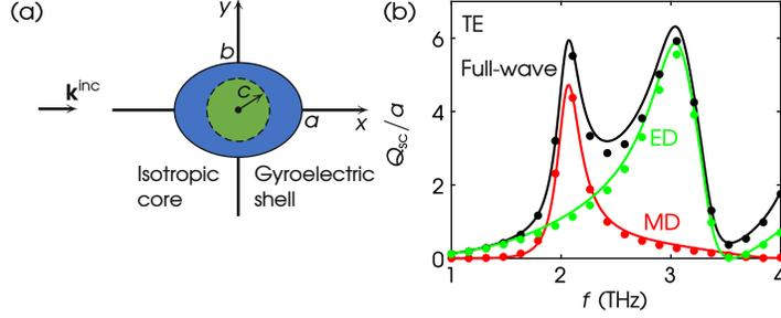
Figure 7: (a) TE scattering by a core-shell circular-elliptical cylinder. Values of parameters:  $\epsilon_{cr} = 25$ ,  $\mu_{cr} = 1$ ,  $\epsilon_{1r} = 4$ ,  $\epsilon_{2r} = 1$ ,  $\epsilon_{3r} = 5$ ,  $\mu_{1r} = 1$ ,  $\mu_{2r} = 0$ ,  $\mu_{3r} = 1$ ,  $a = 20 \mu\text{m}$ ,  $c/a = 0.5$ ,  $b/a = 0.8$ . (b)  $Q_{sc}/a$  spectrum. Curves: MAS; dots: this work via COMSOL; black: full-wave; red: MD; green: ED.
