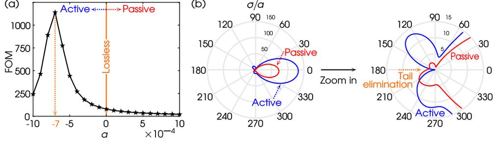
Figure 10: (a) FOM vs.  $\alpha$  for the dimer of Figure 9(a) when  $B_0 = 0.1$  T and  $f = 2.0186$  THz. (b)  $\sigma/a$  at  $\alpha = \mp 7 \times 10^{-4}$ ,  $B_0 = 0.1$  T and  $f = 2.0186$  THz. Blue:  $\alpha = -7 \times 10^{-4}$  (active); red:  $\alpha = +7 \times 10^{-4}$  (passive). Zoom in: tail elimination at back-scattering.
