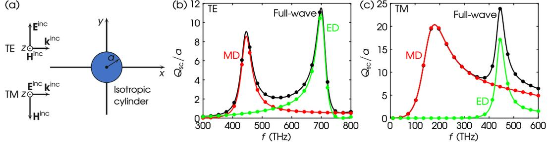
Figure 3: (a) Scattering by an isotropic circular cylinder. Values of parameters:  $\epsilon_{1r} = \epsilon_{3r} = 25$ ,  $\epsilon_{2r} = 0$ ,  $\mu_{1r} = \mu_{3r} = 1$ ,  $\mu_{2r} = 0$ ,  $a = 50$  nm. (b) TE scattering. (c) TM scattering. Curves: exact; dots: this work via COMSOL; black: full-wave; red: MD; green: ED.
