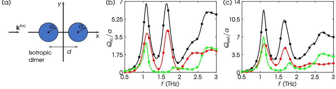
Figure 8: (a) TE scattering by a dimer. Values of parameters:  $\epsilon_r = 25 - i2$ ,  $\mu_r = 1$ ,  $a = 20 \mu\text{m}$ ,  $d = 60 \mu\text{m}$ . (b)  $Q_{sc}/a$  spectrum. Curves: MAS; dots: this work via COMSOL; black: full-wave; red: MD; green: ED. (c) Same as (b) but for  $Q_{ext}/a$ .
