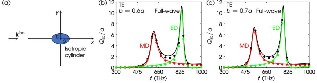
Figure 4: (a) TE scattering by an isotropic elliptical cylinder. Values of parameters:  $\epsilon_{1r} = \epsilon_{3r} = 25$ ,  $\epsilon_{2r} = 0$ ,  $\mu_{1r} = \mu_{3r} = 1$ ,  $\mu_{2r} = 0$ ,  $a = 50$  nm. (b)  $b = 0.6a$ . (c)  $b = 0.7a$ . Curves: Mathieu functions method; dots: this work via COMSOL; black: full-wave; red: MD; green: ED.
