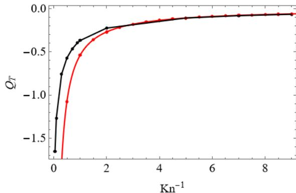
FIG. 3. Normalized flow rate for the thermal creep flow ( $\tau = 1$ ,  $\alpha = 0.5$ ). Solid red line with markers: present rarefied hydrodynamics; Black markers: tabulated numerical calculation for the BGK model [9].
