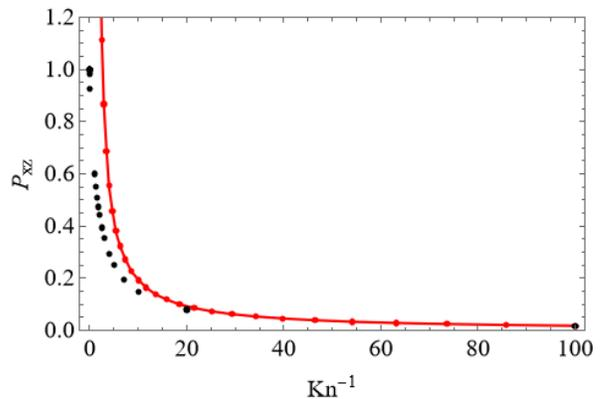
FIG. 2. Normalized stress for the planar Couette flow ( $\tau = 1$ ,  $\alpha = 1$ ). Solid red line with markers: present rarefied hydrodynamics; Black markers: tabulated numerical calculation for the BGK model [9].
