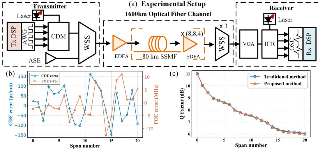
Fig. 5: (a) Experimental setup. (b) CDE and FOE errors of the proposed method. (c) Comparison of Q-factor between the two methods.
