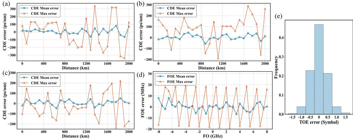
Fig. 4: (a) CDE errors for  $sps = 1$ . (b) CDE errors for  $sps = 1.25$ . (c) CDE errors for  $sps = 2$ . (d) FOE errors for  $sps = 1.25$ . (e) TOE errors for  $sps = 1.25$ .
