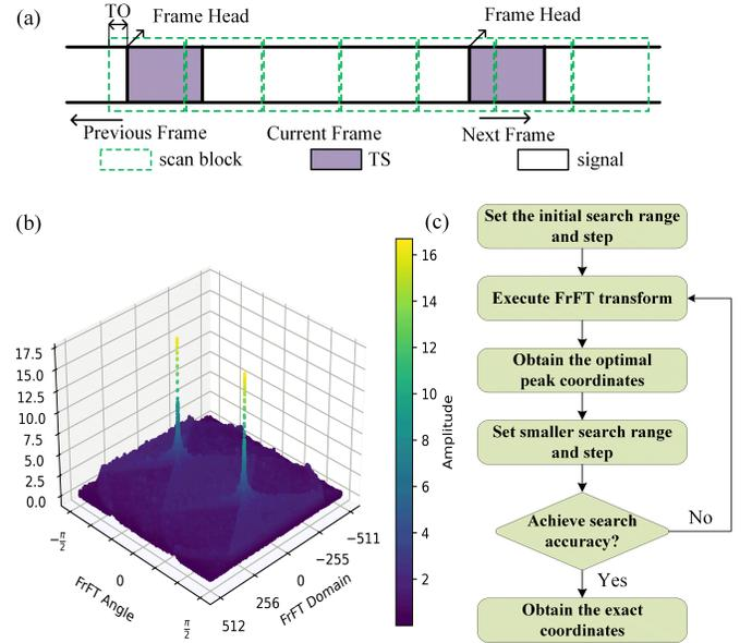
Fig. 2: (a) Coarse framing. (b) FrFT Domain-Angle distribution of TS with  $\alpha = \pi/4$  and  $N_s = 1024$ . (c) Optimal coordinates search flow chart.
