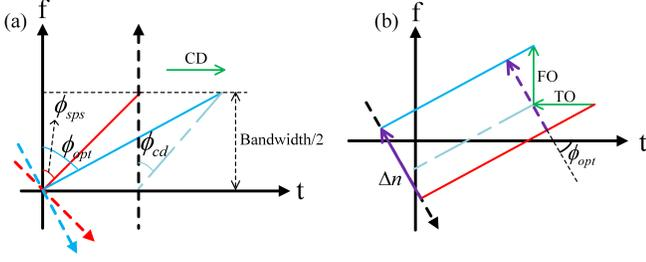
Fig. 1: Time-frequency distribution of chirp signal which is influenced by (a)  $sps$  and CD, (b) TO and FO.
