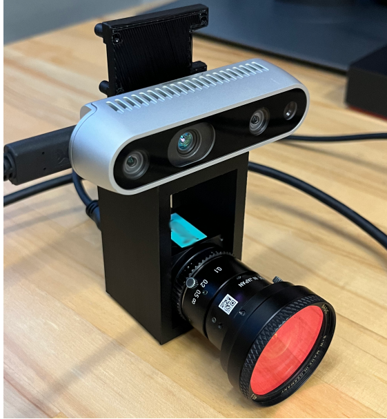
(a) Handheld rig for real-world data collection.
