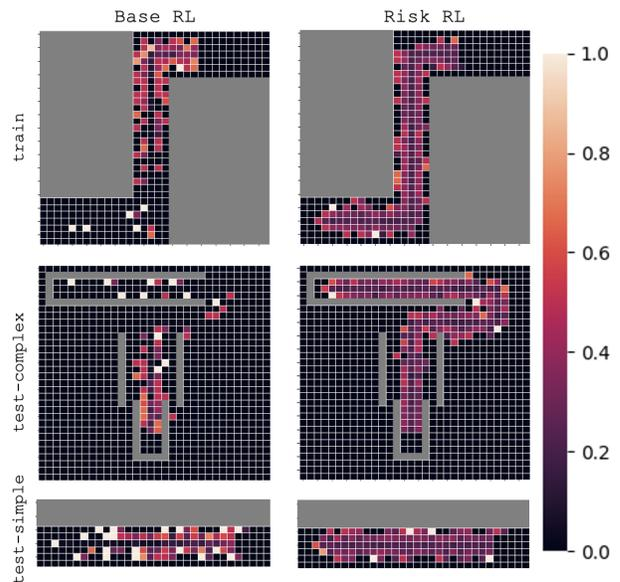
Fig. 8: Probability of localization based on the robot’s estimated location.
