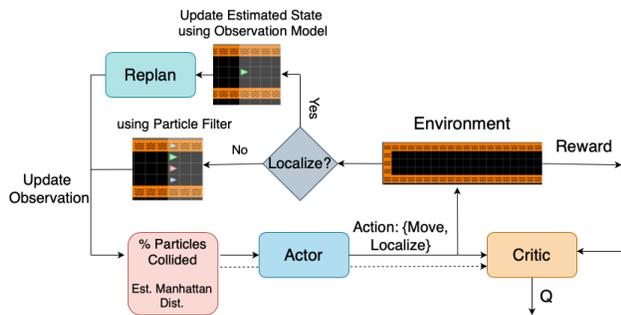
Fig. 2: This flowchart depicts a decision-making process for a robot interacting with an environment. It integrates a particle filter for state estimation and reinforcement learning components (actor-critic architecture) for decision-making.
