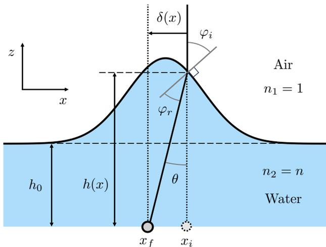
FIG. 4. Ray tracing diagram showing how light rays are refracted through a water layer with an uneven upper surface. The apparent position of a dot is displaced by a distance  $\delta$ , as its image passes through that surface.
