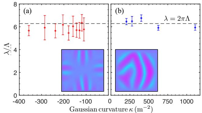
FIG. 9. The characteristic wavelength of the wrinkling of thin curved films agrees with the predictions of elastica-based models [2, 13, 28]. Wavelengths  $\lambda$  are measured for floating films with (a) negative and (b) positive Gaussian curvature  $\kappa$ , as the average distance between successive troughs or peaks of the surface  $h$ , measured on lines parallel to the film's edges. The dashed lines show the prediction that  $\lambda = 2\pi\Lambda$ .
