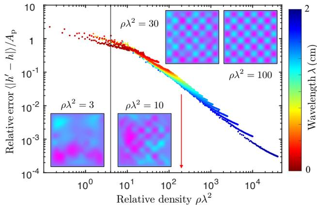
FIG. 5. Surface reconstruction methods were tested with artificial data from a sinusoidal surface. Insets show results for surfaces of width  $W = 4$  cm and wavelength  $\lambda = 1$  cm. The accuracy of the reconstructed surface depends on the relative density of dots used,  $\rho\lambda^2$ . Above the Nyquist condition (solid line,  $\rho\lambda^2 = 4$ ), the relative error improves as  $1/\rho\lambda$ . Our experimental conditions were around  $\rho\lambda \simeq 200$  (red arrow).
