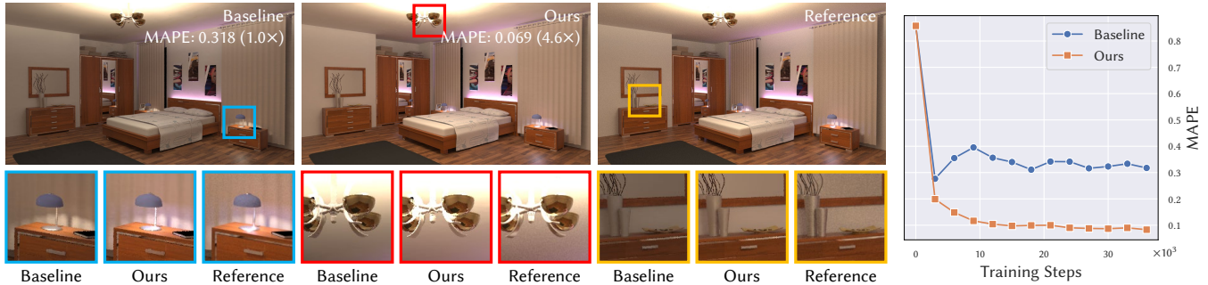
Fig. 1. Rendering residual-based optimization results of the baseline, based on Neural Radiosity [Hadadan et al. 2021], and the proposed method for neural rendering. Previous approaches minimize the L2 distance between the left-hand side (i.e., outgoing radiance) and the right-hand side (i.e., the sum of emitted and reflected radiance) of the rendering equation. We discover that the bias and high variance of the baseline gradient estimator lead to poor convergence, and we propose a partial derivative-based optimization method to resolve them. The graph on the right shows the change in image-space distance from the reference as training progresses.
