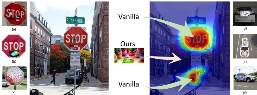
Fig. 1: An illustration of vanilla object attack methods and our novel approach. Typically, vanilla attack methods target the most informative regions of an object, such as the central, highly visible areas of the target object, e.g., the stop sign in (a) [16], (b) [67], (c) [15], and the car in (d) [19], (e) [57], (f) [22]. In contrast, our method adopts a more covert strategy, focusing on attacking the peripheral edge areas surrounding the stop sign.
