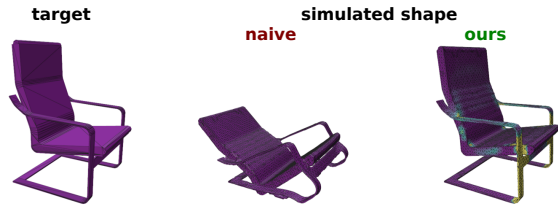
Fig. 13. Optimizing the stability such that the chair remains stable to a force applied on the backrest. From left to right, reconstructed shape without (naive) then with (ours) physics-aware loss, simulated reconstruction without (naive) then with (ours) physics-aware loss. The yellow ball on the rest geometries indicates the position of the center of mass.
