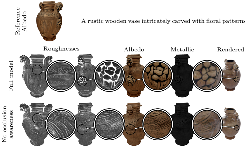
Fig. 8: Ignoring occlusions in the masked attention from Fig. 5 results in features leaking towards back views, most noticeably from the reference view.
