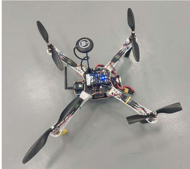
Figure 3: Quadrotor platform used for flight data gathering, with one damaged propeller.
