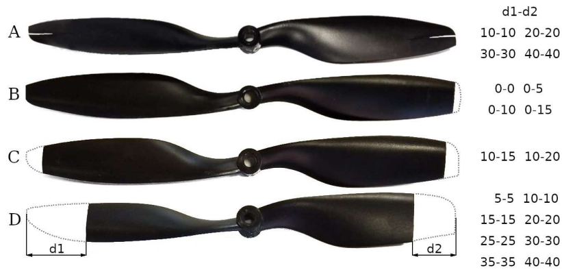
Figure 1: Propellers with, A-longitudinal, B,C-asymmetrical, and D-symmetrical damages. The numbers on the right indicate the cuts performed on each of the 18 propellers used
