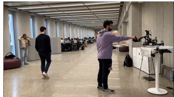
Fig. 1. Our robot is tested in two different public environments: it must track multiple nearby people, predict their intention to interact, and proactively offer them chocolate treats.
