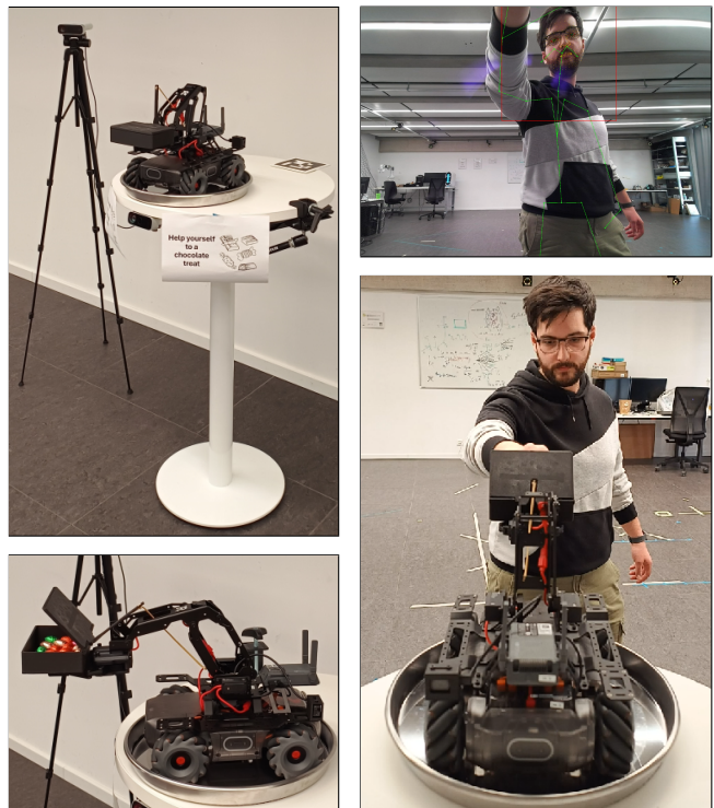
Fig. 2. Experimental setup (top left) with a zoomed view of the robot with the stretched arm offering chocolate treats (bottom left); a view from behind the robot interacting with a user (bottom right), and the same situation captured by the Robot Sensor (top right).
