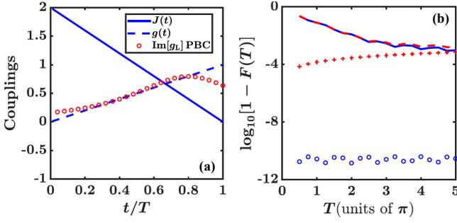
FIG. 3. W-state generation. (a) Couplings  $J(t)$ ,  $g(t)$ , and  $\text{Im}[g_L]$  for  $T = 0.5\pi$ . (b) Infidelity  $1 - F(T)$  vs  $T$ . The solid (dashed) line is for  $\kappa = \gamma = 0$  ( $\kappa = 5 \times 10^{-5}$  and  $\gamma = \frac{5}{\pi} \times 10^{-5}$ ) under  $H_r$  only; and circles (crosses) are for  $\kappa = \gamma = 0$  ( $\kappa = 5 \times 10^{-5}$  and  $\gamma = \frac{5}{\pi} \times 10^{-5}$ ) when  $H_L$  is applied. All parameters are in dimensionless units.
