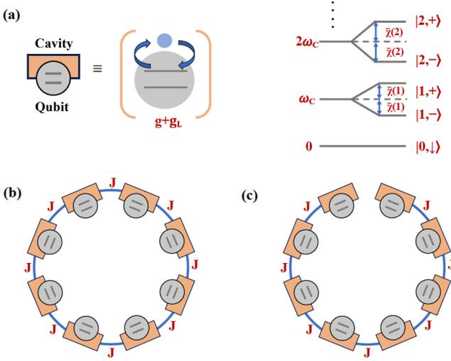
FIG. 1. (a) Schematic of a JC model (left) and its eigenstates (right). Here  $g$  is the qubit-cavity coupling strength,  $g_L$  is the strength of the local CD driving, and  $\bar{\chi}(n)$  is the energy splitting of the eigenstates with  $n$  excitations. (b) and (c) JC lattices under periodic and open boundary conditions respectively, with photon hopping rate  $J$ .
