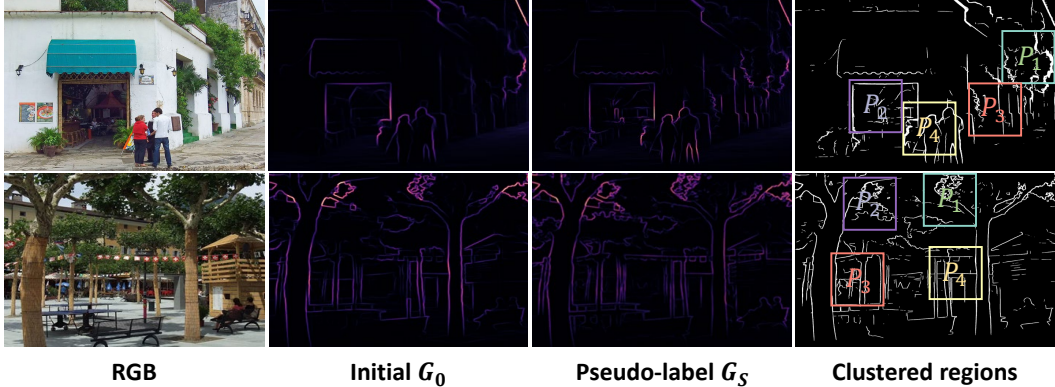
Figure 10: Edge-guided gradient error. \mathcal{L}_{grad} focuses on high-frequency areas P_n extracted by clustering with more details. The flat regions are not constrained to preserve depth consistency.
