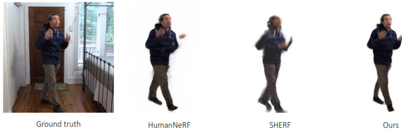
Fig. 10: Qualitative comparison for learning a novel identity. From left to right: ground truth, results of HumanNeRF [64], SHERF [25], and our multi-identity model. Our method robustly renders the new identity under completely unseen poses, given only a very short video of 10 seconds.
