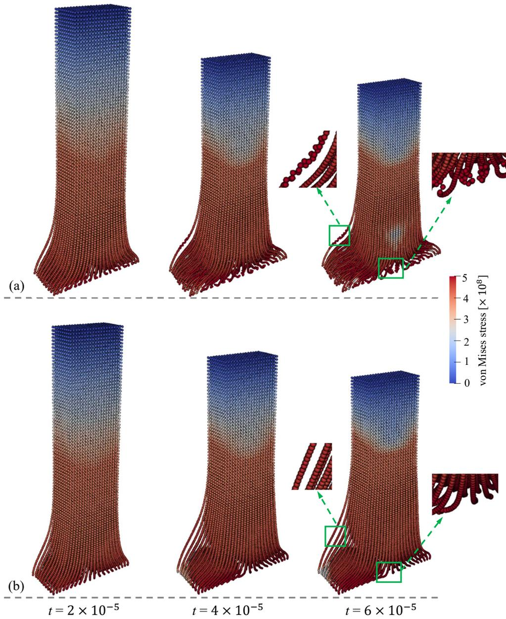
**Fig. 25.** Square Taylor bar: evolution of particle configuration with time. The results are obtained by (a) SPH-OG and (b) the present SPH-GNOG. The initial particle spacing  $dp = W/20$  and the particles are colored by von Mises stress.
