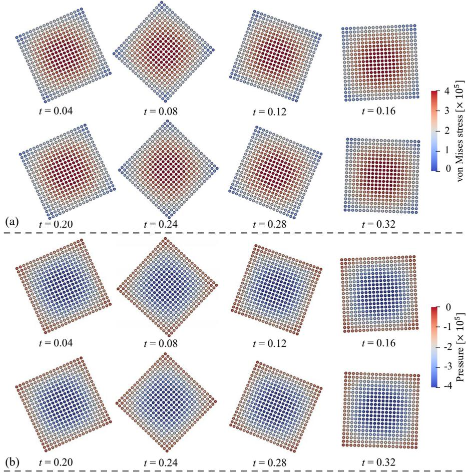
**Fig. 18.** Spinning plate: the evolution of particle configuration at different instants. The particles are colored by (a) von Mises stress and (b) pressure respectively.
