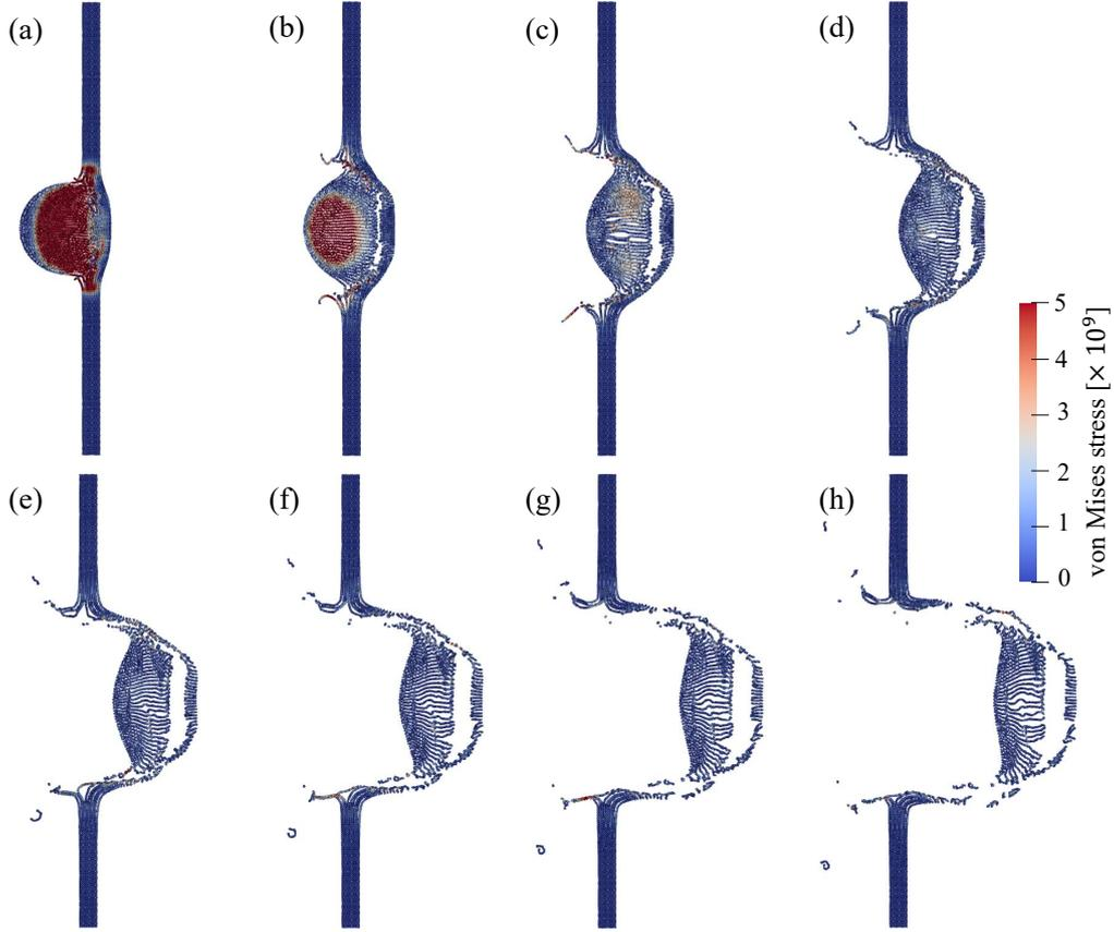
**Fig. 28.** High-velocity impact: evolution of von Mises stress with the present SPH-GNOG at (a)  $t = 1 \times 10^{-6}$ , (b)  $t = 2 \times 10^{-6}$ , (c)  $t = 3 \times 10^{-6}$ , (d)  $t = 4 \times 10^{-6}$ , (e)  $t = 5 \times 10^{-6}$ , (f)  $t = 6 \times 10^{-6}$ , (g)  $t = 7 \times 10^{-6}$ , (h)  $t = 8 \times 10^{-6}$ .
