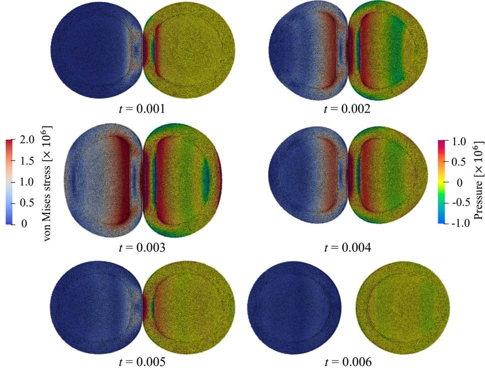
**Fig. 15.** 3D colliding rubber balls: evolution of particle configuration with time. The results are obtained by the present SPH-GNOG. The initial velocity magnitude  $v_0 = 0.08c_0$ . The left ball is colored by von Mises stress, and the right ball is colored by pressure.
