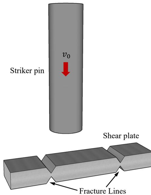
**Fig. 30.** Striker pin fuse: model setup.
