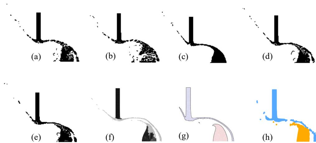
**Fig. 29.** High-velocity impact: deformation of projectile and target at  $t = 8 \times 10^{-6}$  obtained with different algorithms, i.e., (a) BAL [60], (b) MON [60], (c) CON [60], (d) SAV1 [60], (e) SAV2 [60], (f) adaptive total Lagrangian Eulerian SPH [61], (g) Xiao and Liu's study [66], (h) the present SPH-GNOG.
