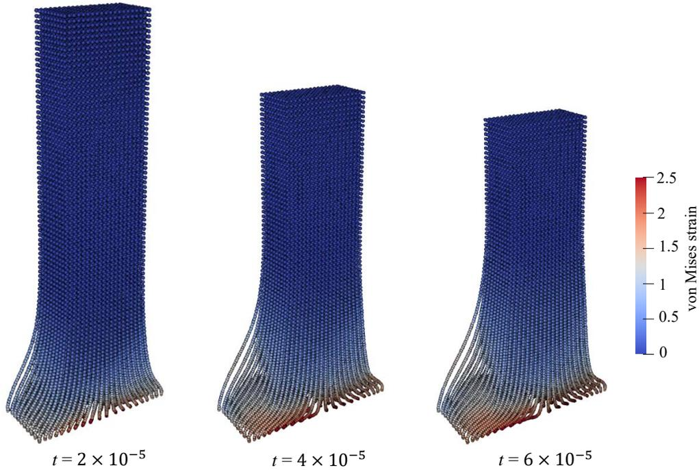
**Fig. 26.** Square Taylor bar: evolution of von Mises strain with the present SPH-GNOG. Here,  $dp = W/20$ .
