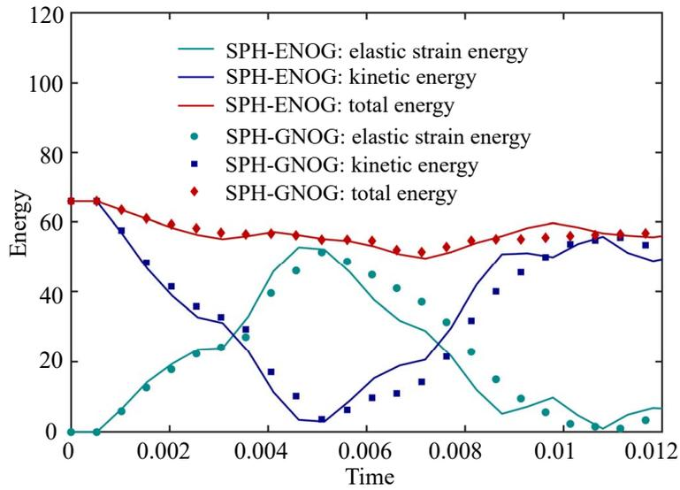
**Fig. 14.** 2D colliding rubber rings: the variation of elastic strain energy, kinetic energy, and total energy over time for the left ring with the SPH-ENOG [24] (represented by solid lines) and SPH-GNOG (represented by dots). The initial velocity magnitude  $v_0 = 0.06c_0$ .
