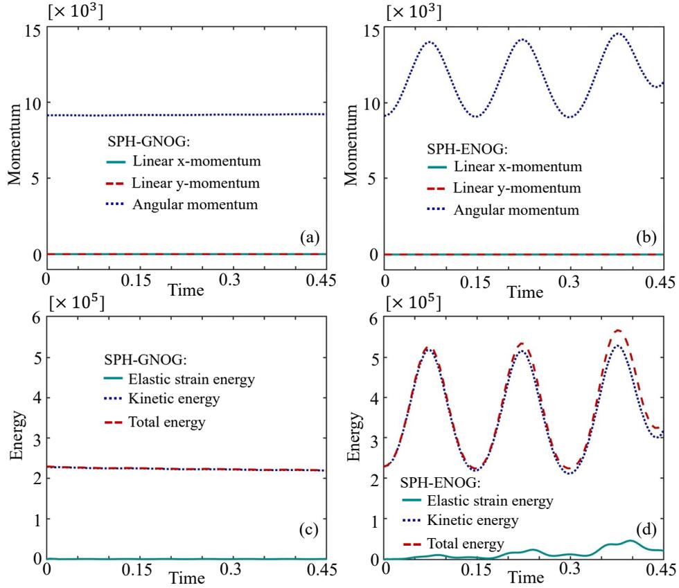
**Fig. 20.** Spinning plate: the temporal evolution of the system’s momentum and energy SPH-GNOG and SPH-ENOG. (a) The total linear momentum and angular momentum with SPH-GNOG; (b) the total linear momentum and angular momentum with SPH-ENOG [24]; (c) the elastic strain energy, kinetic energy and total energy with SPH-GNOG; (d) the elastic strain energy, kinetic energy and total energy with SPH-ENOG [24].
