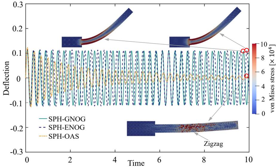
**Fig. 5.** 2D oscillating plate: test the long-time stability of the SPH-GNOG. The result is compared with those obtained by SPH-ENOG [24] and SPH-OAS [24]. Here,  $L=0.2$ ,  $H=0.02$ ,  $H/dp = 10$  and  $v_f=0.05$ . The particles are colored by von Mises stress.
