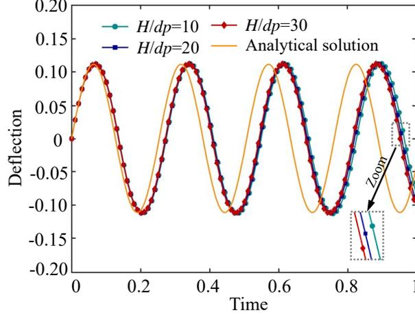
**Fig. 3.** 2D oscillating plate: temporal evolution of deflection at various resolutions. Here,  $v_f = 0.05$ ,  $L = 0.2$ , and  $H = 0.02$ .
