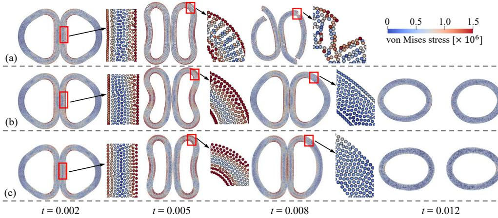
**Fig. 13.** 2D colliding rubber rings: evolution of particle configuration with time ( $t = 0.002, 0.005, 0.008$  and  $0.012$ ). The results are obtained by three different SPH strategies, i.e., (a) SPH-OAS [24], (b) SPH-ENOG [7, 24], and (c) SPH-GNOG. The initial velocity magnitude  $v_0 = 0.08c_0$  and the particles are colored by von Mises stress.
