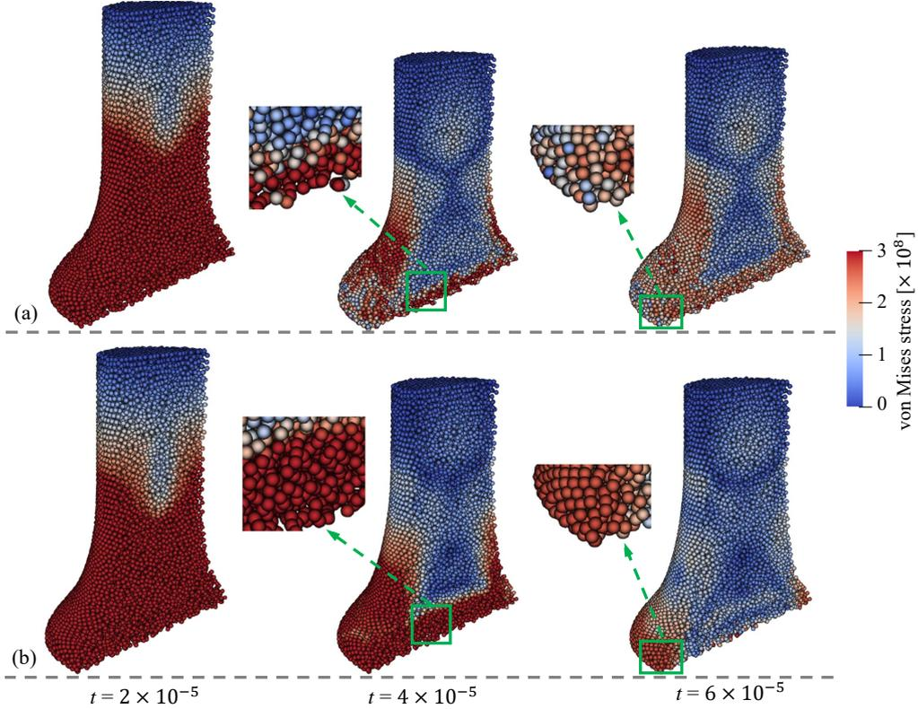
**Fig. 22.** Round Taylor bar: evolution of particle configuration with time. The results are obtained by (a) SPH-OG and (b) SPH-GNOG. The initial particle spacing  $dp = R/12$  and the particles are colored by von Mises stress.
