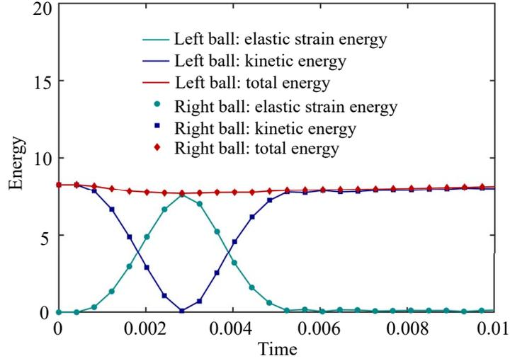
**Fig. 16.** 3D colliding rubber balls: the variation of elastic strain energy, kinetic energy, and total energy over time for the left (represented by solid lines) and right (represented by dots) balls. The initial velocity magnitude  $v_0 = 0.08c_0$ .
