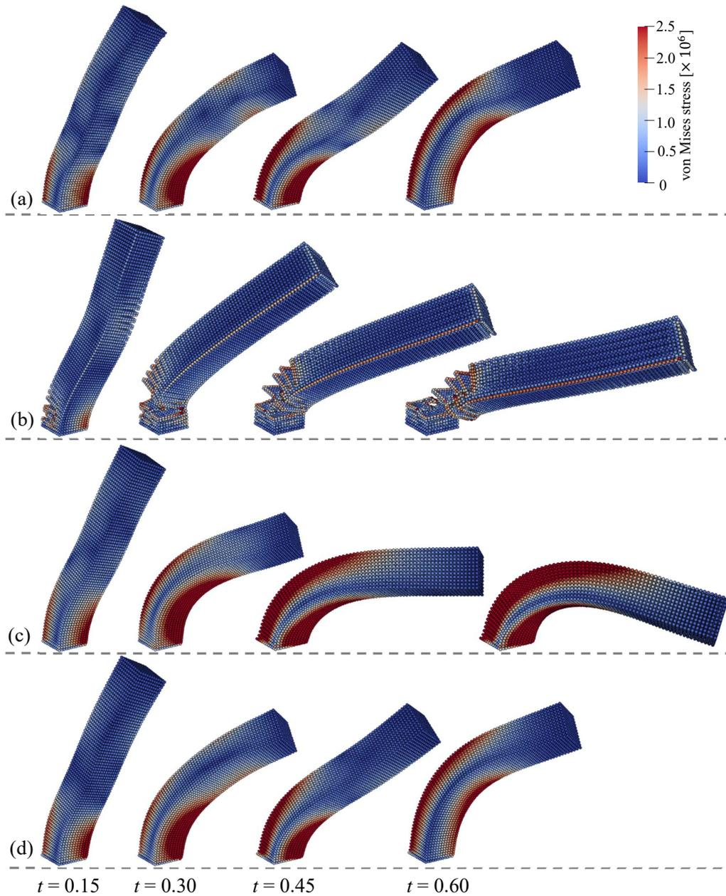
**Fig. 7.** 3D bending column: evolution of particle configuration with time ( $t=0.15, 0.30, 0.45$  and  $0.60$ ) for (a) TLSPH [30], (b) SPH-OG, (c) SPH-ENOG [24], and (d) SPH-GNOG. Here,  $L/dp = 12$  and  $dp$  is the initial particle spacing. The particles are colored by von Mises stress.
