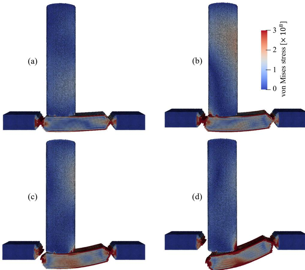
**Fig. 31.** Striker pin fuse: evolution of von Mises strain with the present SPH-GNOG at (a)  $t = 1 \times 10^{-5}$ , (b)  $t = 2 \times 10^{-5}$ , (c)  $t = 4 \times 10^{-5}$ , (d)  $t = 1 \times 10^{-4}$ .
