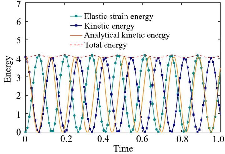
**Fig. 4.** 2D oscillating plate: temporal evolution of elastic strain energy, kinetic energy, and total energy. Here,  $v_f = 0.05$ ,  $L = 0.2$ , and  $H = 0.02$ .
