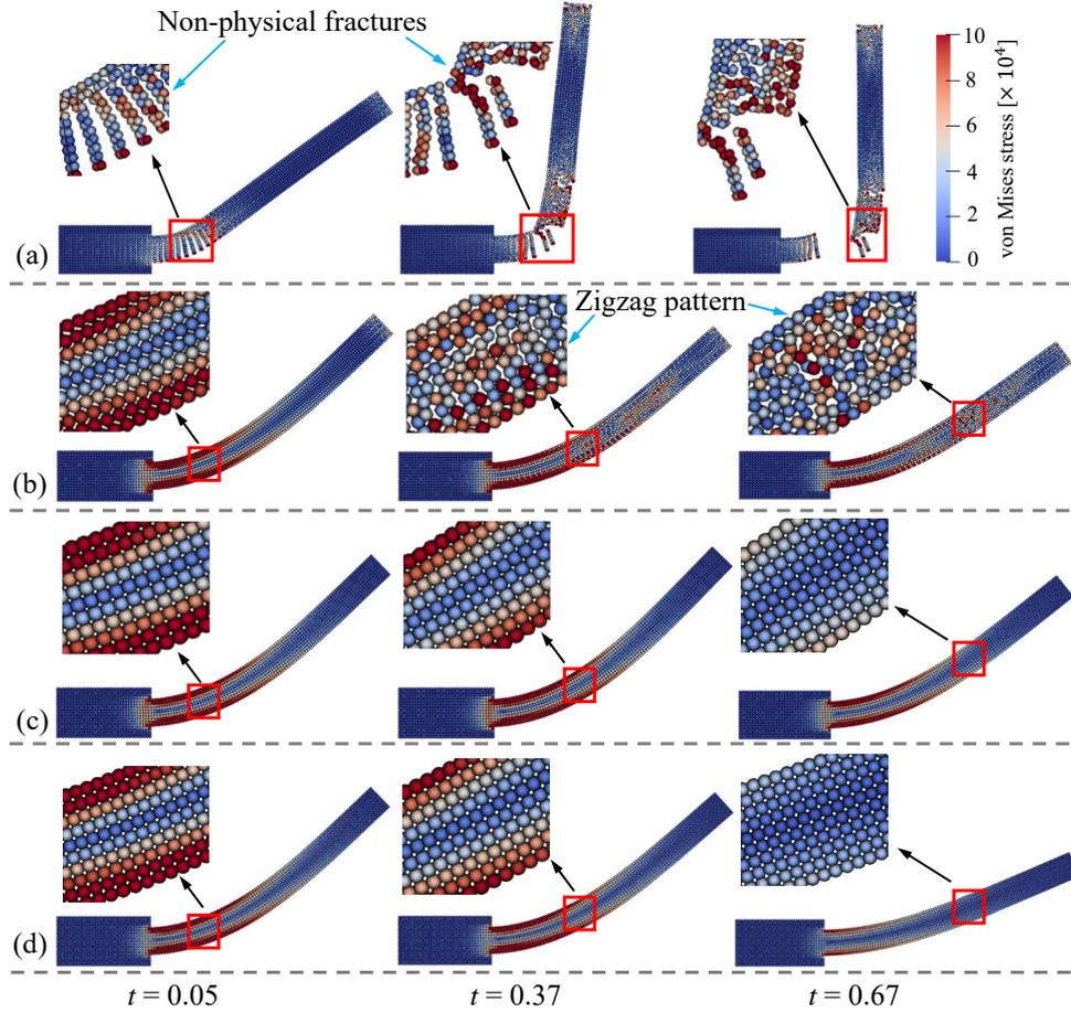
**Fig. 2.** 2D oscillating plate: evolution of particle configuration with time ( $t=0.05$ ,  $0.37$  and  $0.67$ ) for (a) SPH-OG [24], (b) SPH-OAS [7, 24], (c) SPH-ENOG [24], and (d) SPH-GNOG. Here,  $v_f = 0.05$ ,  $L = 0.2$ , and  $H = 0.02$ . The particles are colored by von Mises stress.
