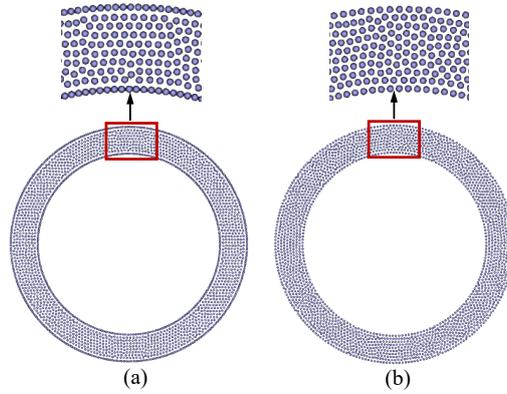
**Fig. 11.** 2D colliding rubber rings: initial particle distribution in the study of Zhang et al. [24] and (b) this study.
