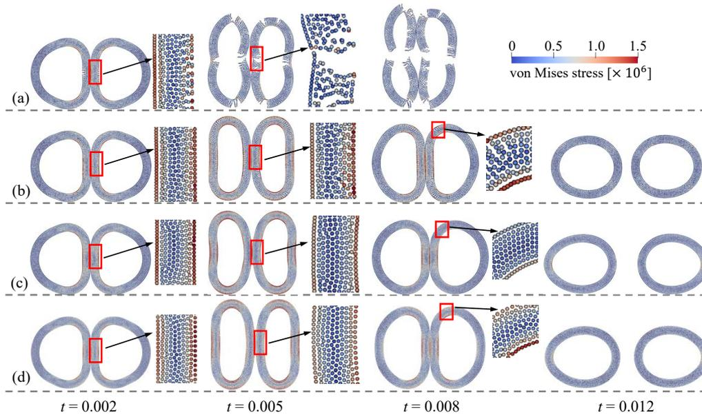
**Fig. 12.** 2D colliding rubber rings: evolution of particle configuration with time ( $t = 0.002, 0.005, 0.008$  and  $0.012$ ). The results are obtained by four different SPH strategies, i.e., (a) SPH-OG [24], (b) SPH-OAS [7, 24], (c) SPH-ENOG [24], and (d) SPH-GNOG. The initial velocity magnitude  $v_0 = 0.06c_0$  and the particles are colored by von Mises stress.
