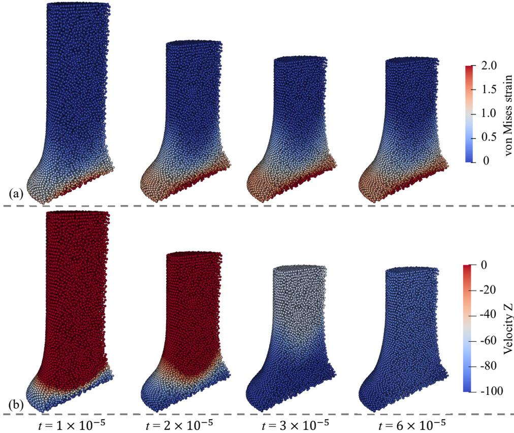
**Fig. 23.** Round Taylor bar: evolution of (a) von Mises strain and (b) z-component of velocity with the present SPH-GNOG. Here,  $dp = R/12$ .
