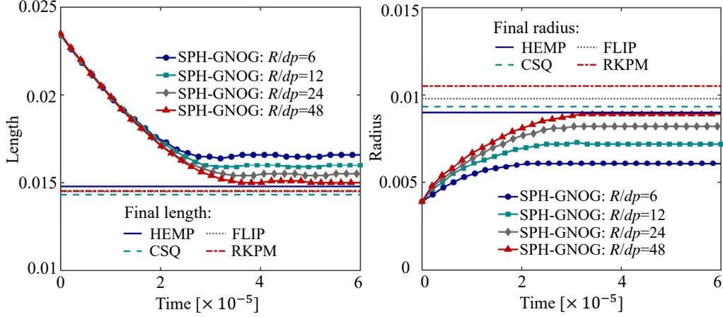
**Fig. 24.** Round Taylor bar: temporal evolution of length and radius of the bar at various resolutions. The results are compared with the final values of length and radius obtained from HEMP [55], CSQ [56], FLIP [57], and RKPM [53].
