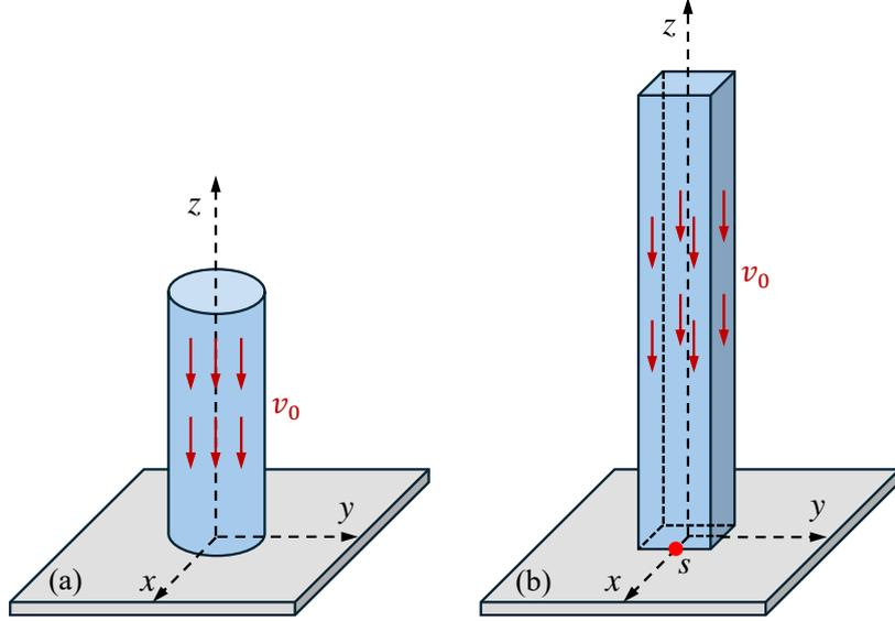
**Fig. 21.** Model setup for (a) round Taylor bar and (b) square Taylor bar.
