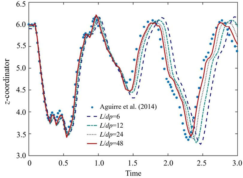
**Fig. 9.** 3D bending column: time history of the vertical position  $z$  observed at node  $s$  obtained by SPH-GNOG with for different spatial resolutions. The results are compared with those obtained with FVM by Aguirre et al. [49]
