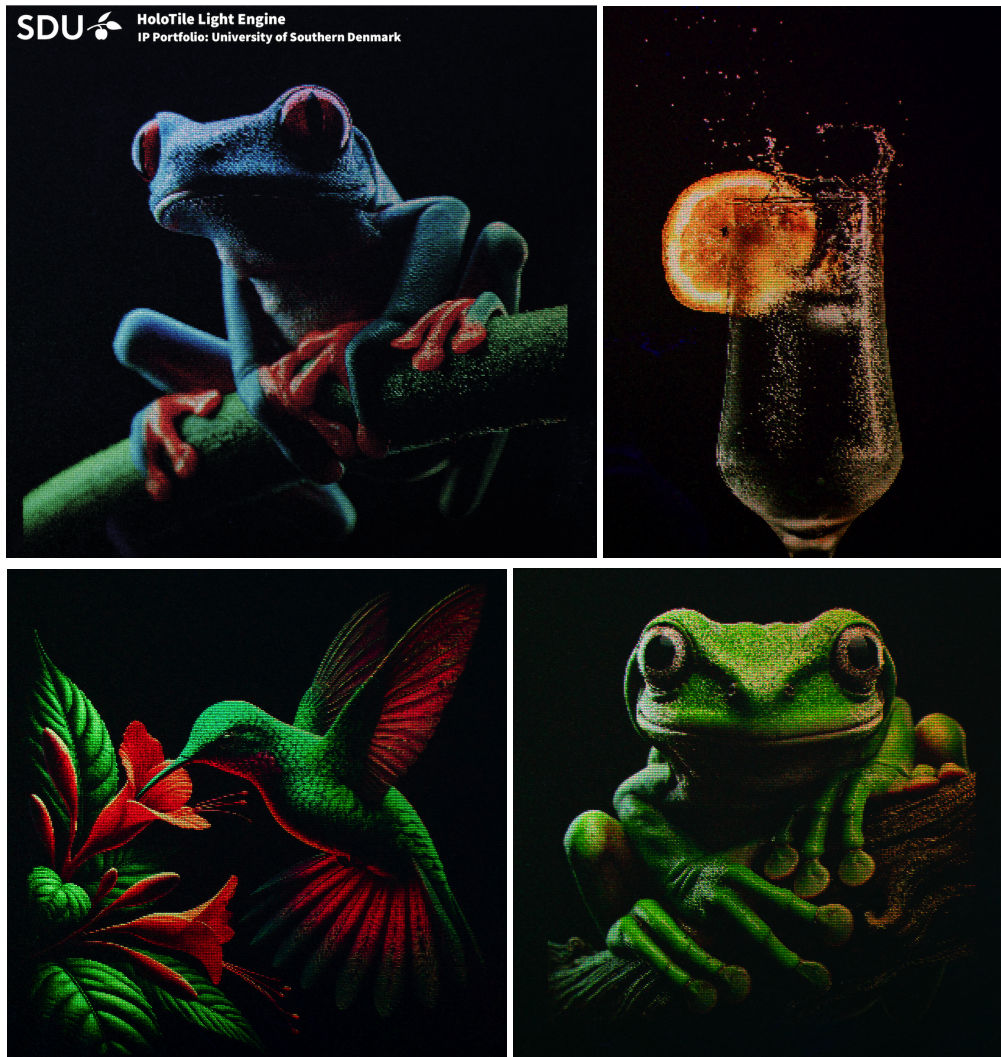
Fig. 7. Lensed experimental targets captured directly in camera in a single shot without temporal averaging. Holograms are added a linear phase to filter out the zero order.
