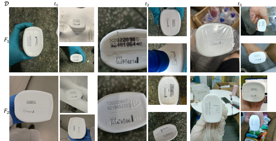
Fig. 2: Sample images of the bottom side of commercial products produced by two factories, F_1 and F_2 , in three temporally continuous datasets, i.e. \mathcal{D}_{t_1} , \mathcal{D}_{t_2} and \mathcal{D}_{t_3} . The ACF code is the region of interest required to be segmented and cropped.
