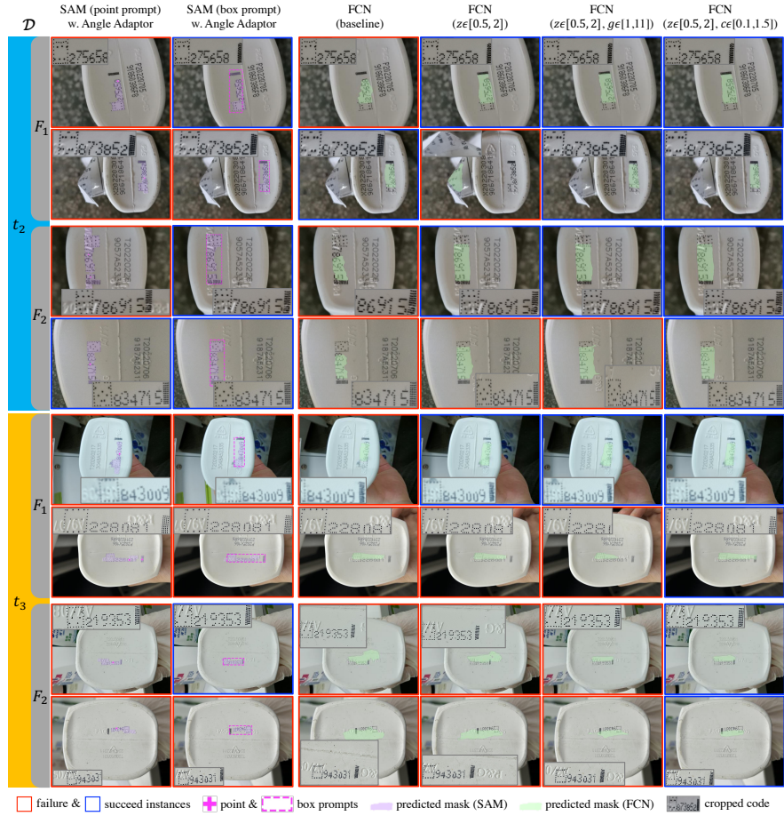
Fig. 4: Detailed comparisons of segmentation and cropping among pre-trained SAM and FCN baseline where our proposed ARMF framework is applied.
