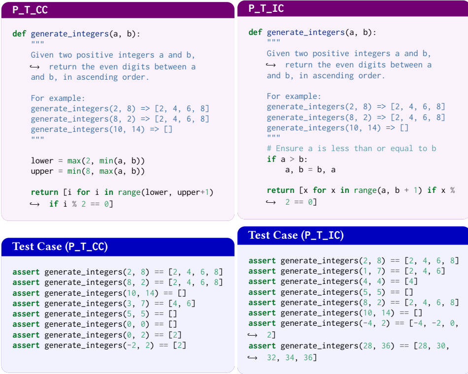
Fig. 4. Example of prompt-based and completed-code-based test case generation by GPT-4-turbo. The prompt provides a function skeleton to generate even integers between two given numbers. When generating test cases directly from the prompt, the GPT-4-turbo correctly focuses on the digits (0-9). In contrast, when generating test cases from the completed code, GPT-4-turbo considers numbers beyond the digit range (e.g., 28 and 36), illustrating that the incorrect code affects the test case accuracy when we feed the completed code into the GPT-4-turbo.
