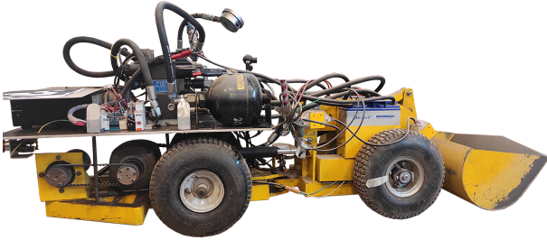
Fig. 11. Side view of the scaled LHD used for real world experiments.
