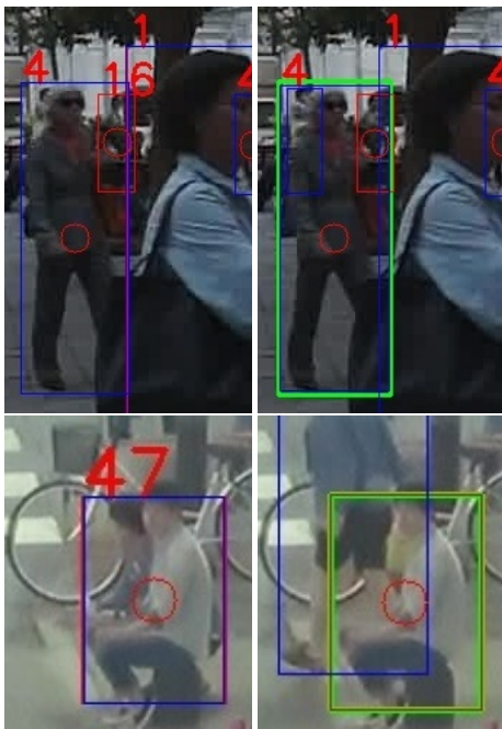
Figure 5. Some cases where erroneous candidacy of a tracklet is caught and thresholded by aspect ratio similarity. Blue boxes are detections, red boxes are tracklets and the green boxes are the tracklets that were decided to be candidates for multiple or wrong detections, but avoided by ARS thresholding.
