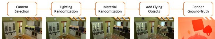
Fig. 5: Synthetic dataset generation pipeline. We perform these steps to boost the frequency of non-Lambertian object appearances and the diversity of rendered images.
