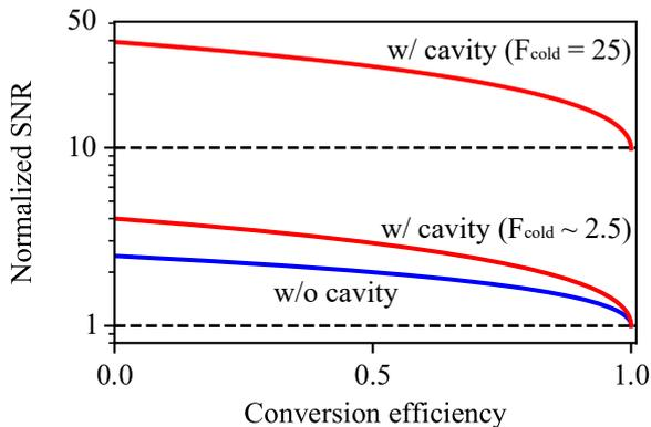
FIG. 4. Normalized SNR v.s. conversion efficiency. The normalization is based on taking the value of  $SNR_{\text{nocav}}$  at  $\eta_{\text{nocav}} = 1$  by using  $B/\alpha_{\text{noise}} = \pi^2/4 \sim 2.5$ . Blue: conventional QFC. Red: cavity-enhanced QFC with  $F_{\text{cold}} = 8/\pi \sim 2.5$  and 25.
