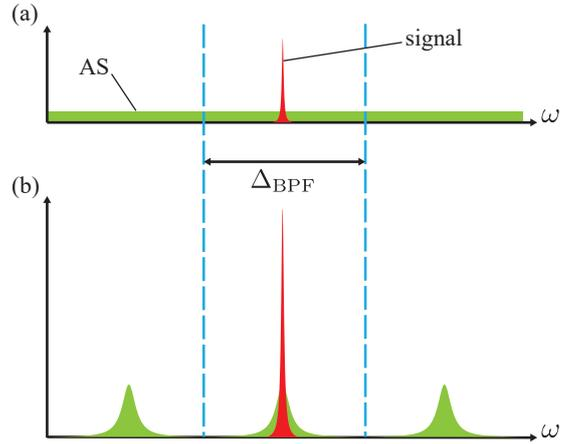
FIG. 3. The spectrum of signal and AS photons (a) without and (b) with a cavity. The total amounts of AS photons within the range of FSR are the same when the pump powers used for both cases are equal.
