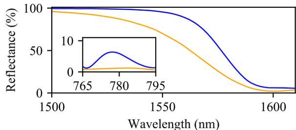
FIG. 10. The data of the reflectance of the front (blue) and rear (orange) sides of the PPLN-WR.
