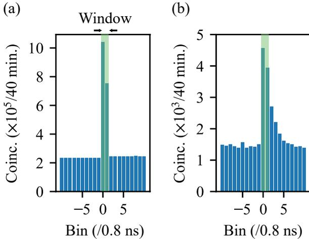
FIG. 8. (a) Observed coincidence counts in 40 minutes between the signal and idler photons. (b) Observed coincidence counts in 40 minutes between the converted and idler photons with  $P \sim 140$  mW. The time resolution and width of the window are 0.8 ns and 1.6 ns.
