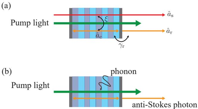
FIG. 2. Theoretical model of (a) the frequency conversion in the cavity and (b) the generation of AS photons.
