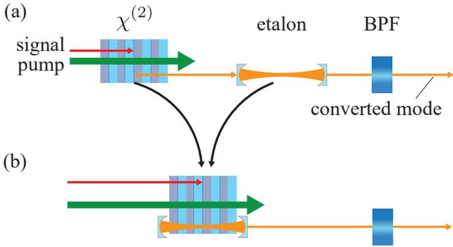
FIG. 1. (a) Conventional QFC system and (b) our QFC system
