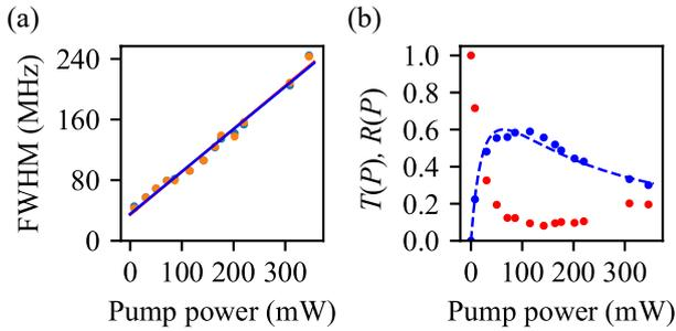
FIG. 11. (a) Pump power dependencies of observed bandwidths of transmitted (red) and converted (blue) light for the 1600 nm. (b) Pump power dependencies of  $T(P) = |t_{ss}|^2$  (red) and  $R(P) = |r_{rs}|^2$  for  $\tilde{\Delta} = 0$ . The blue dashed line was obtained from Eq. (2) using  $(\tilde{\alpha}^{\text{ex}})^{-1} \sim 61$  mW and  $\tilde{\gamma}_r = 0.7$ .
