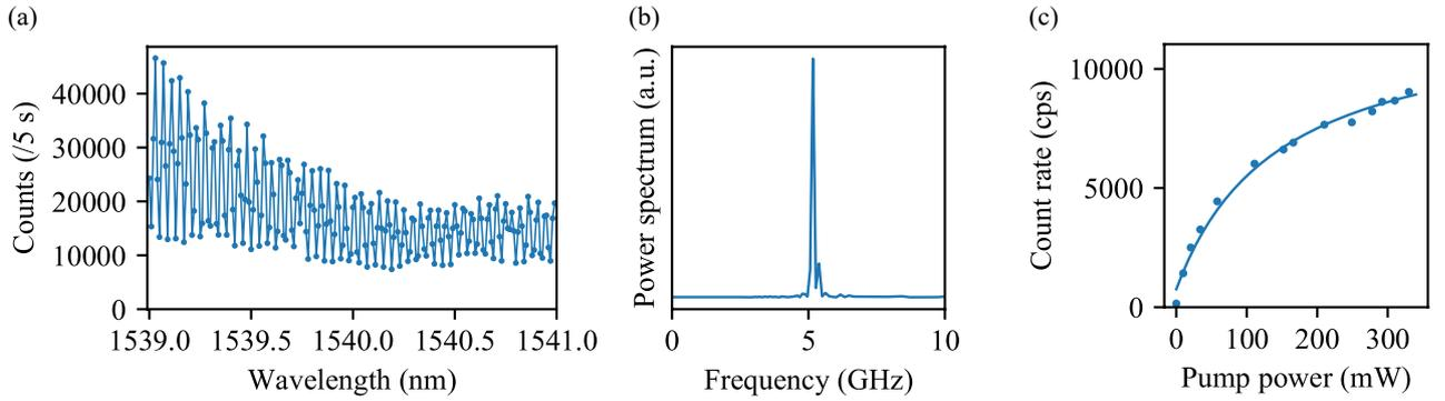
FIG. 7. (a) Photon count distribution of AS photon around 1540 nm. (b) The power spectrum of AS photons obtained by performing the Fourier transform to the data (a). (c) The pump power dependency of the number of AS photons. The blue line is calculated using Eq. (D5) and the data of bandwidths of 1540 nm converted light.
