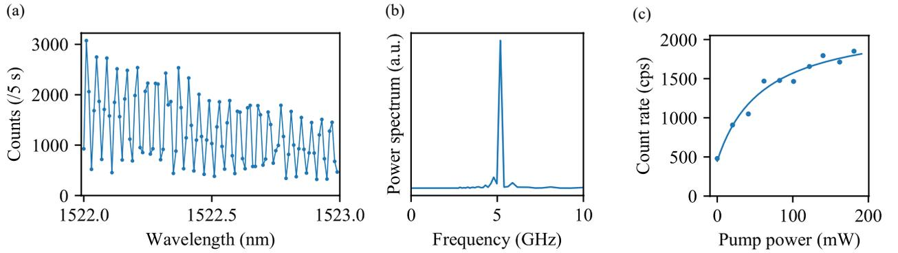
FIG. 12. (a) Photon count distribution of AS photon around 1522 nm and (b) its power spectra. (c) The pump power dependency of the number of AS photons. The blue line is calculated using Eq. (D5) and the data of bandwidths of 1522 nm converted light.
