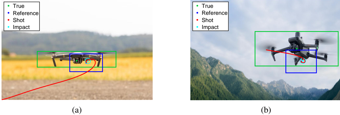
Figure 4: Example output from two targeting simulations. Note, the images are not part of the dataset used to train the object detection model, but are publicly available. In (a), targeting starts from the bottom left corner of the image and in (b), targeting starts from the center of the image.
