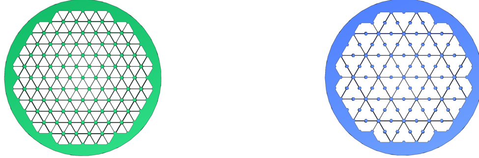
(a) Top view of a framed arrangement; full web with 1.5 mm walls (b) Top view of a semi-frameless arrangement; partial web with 1.5 mm walls
