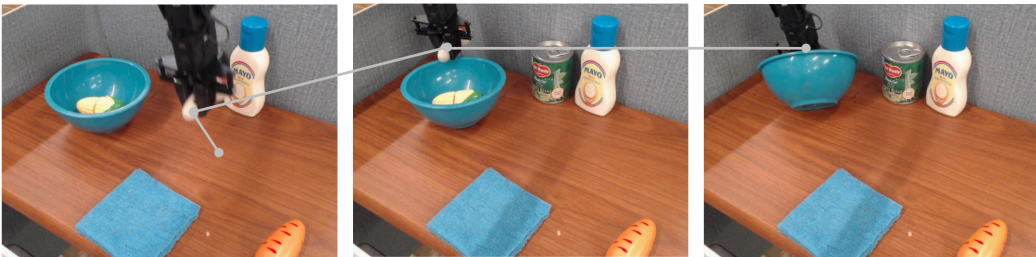
Figure 10: Grounding failure occurred when high level instruction is masked out. While the low level instruction “move the gripper left” correctly predicts the next reasonable action, masking out the context of the subtask “put the mushroom in the bowl” causes the policy to overshoot its trajectory.
