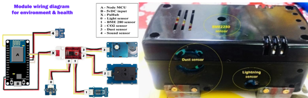
Figure 2a and 2b. Schematics for environmental sensors device and assembled device.
