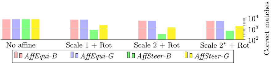
**Fig. 4:** Measuring the affine steering capabilities of the different descriptors. We count correct matches when using the steerer with the ground truth affine map on affinely augmented images. We vary the affine maps by scale. “+ Rot” means that all inplane rotations are included. “Scale 2\*” means that the scale of the affine map  $M$  is maximum 2, but the matrix that is fed to the steerer is  $M/\sqrt{\det M}$  and so has determinant 1.
