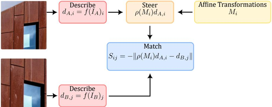
**Fig. 2: Overview of the steering idea for keypoint matching.** An affine steerer gives a way to modify descriptions as if they were obtained from warped images, without having to rerun the descriptor network on warped images. The steerer is a linear map and hence computationally light to use.
