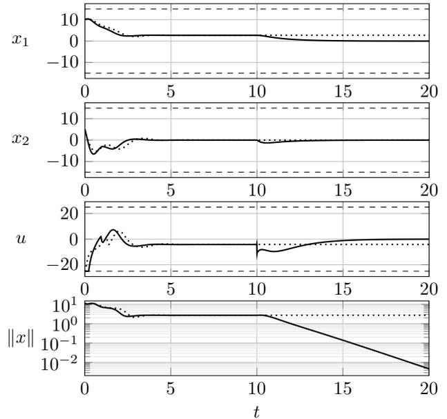
Fig. 1: Closed-loop results of the proposed MPC controller (—) with input constraints (---), where we switch to the terminal control law after  $t = 10$ . MPC results for a linear Koopman surrogate model (····) are included for comparison.
