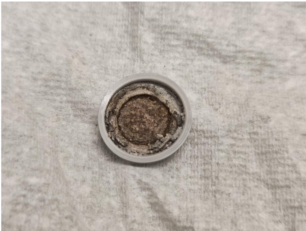
Figure S22 Sodium anode after overcharging in a NVPC/CNTF half-cell with 60.7 \text{ mg cm}^{-2} areal loading, 20 cycles in total.
