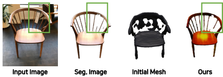
Figure S21: Limitation of model dependencies. The green square indicates object occlusion in the input image, which disrupts segmentation, leading to the disappearance of the reconstruction mesh.
