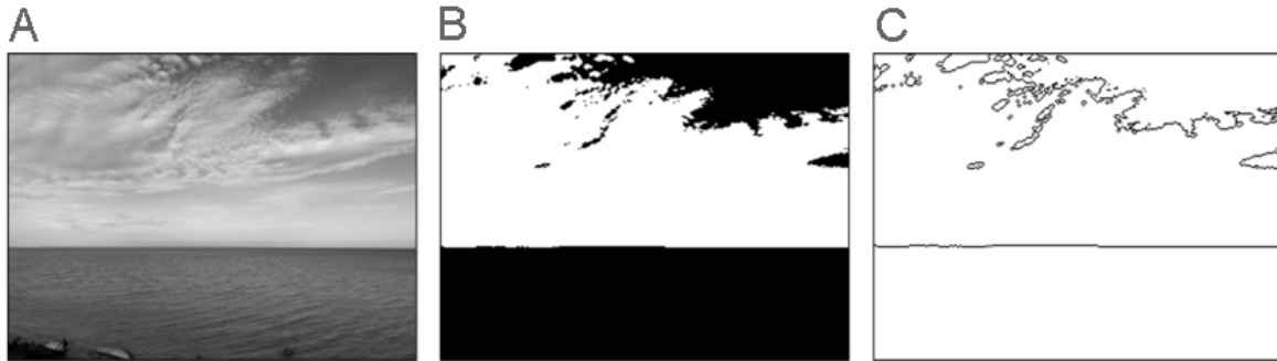
Figure 5: Original grayscale image (A), thresholded image (B), and edges-only image (C).
